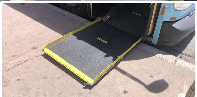
Regular ADA ramp provided at front door.
