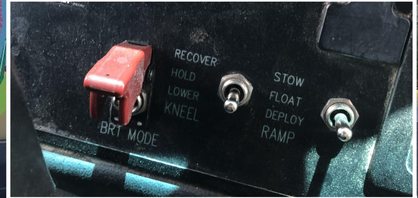
"BRT Mode" increases ride height when flashers are on and governs speed (e.g. 35mph).
