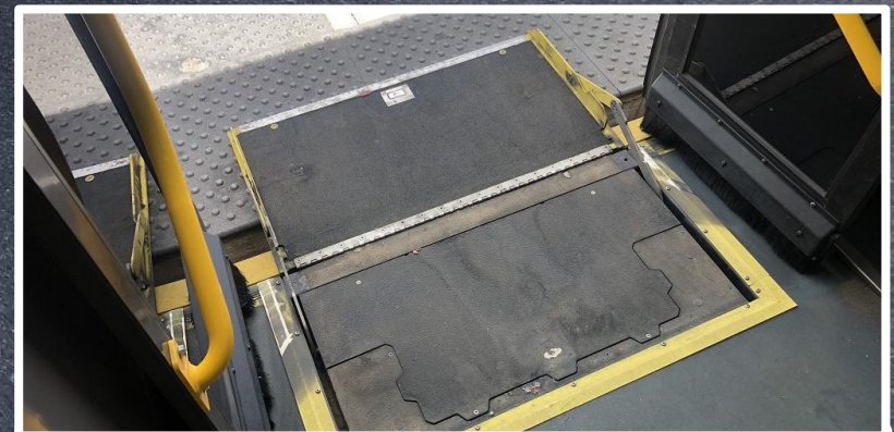
Rear and middle doors have driver operated ramps.
