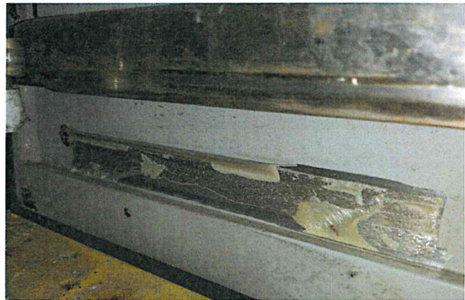
Image 15: Bonding area of kick out protection on left door leaf of doorway #1 vehicle 316
