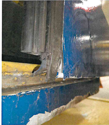
Image 17: Plastic deformation on left door leaf
